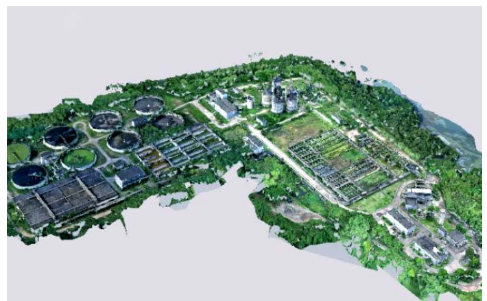
Leveraging ContextCapture, Aegea processed 156,000 drone-captured photos in record time, generating 3D digital twins.
