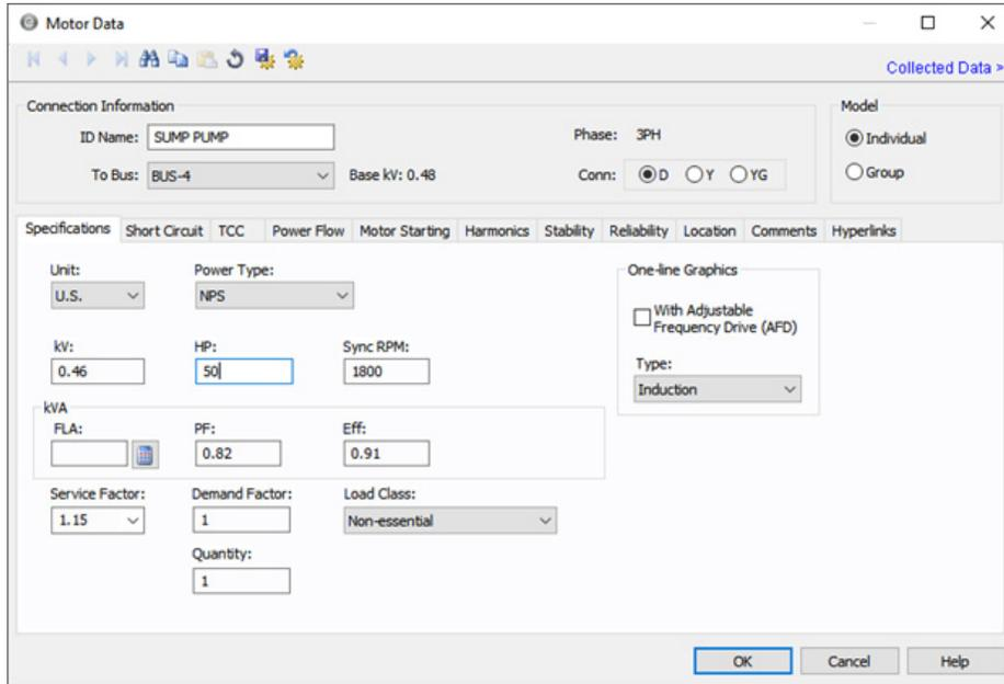
Figure 8.16: Data Entered in the Motor Specification Tab
