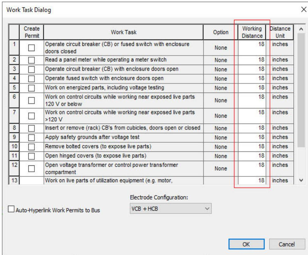
Figure 3.4 – Working Distance, Within the Energized Work Permit dialogue box
