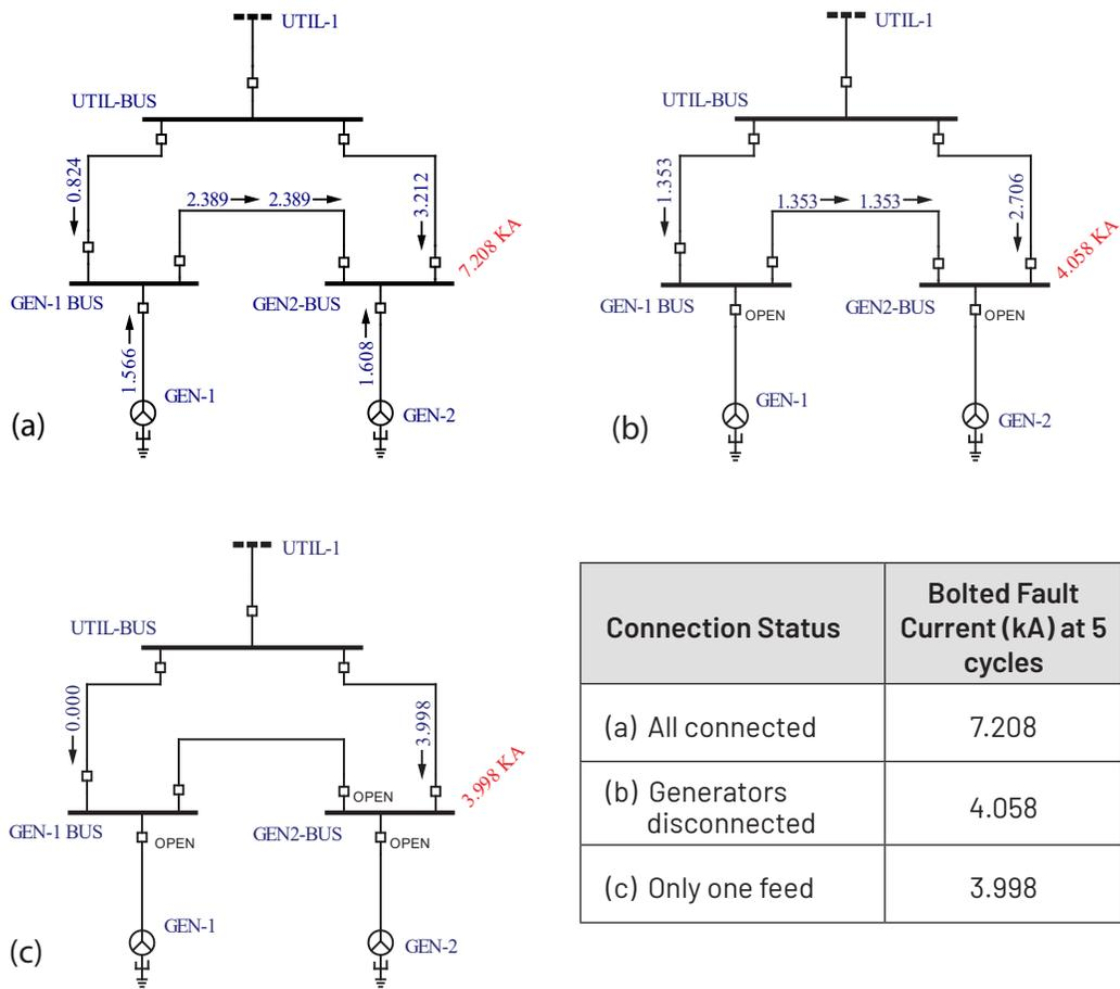
Figure 4.4: Example Showing a Multiple Source Fed Bus Fault and the Series of Operations with the Fault Current Changing with the Breaker Operation
