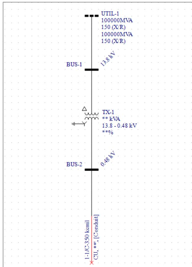
Figure 8.8: Cable Connected to the Transformer
