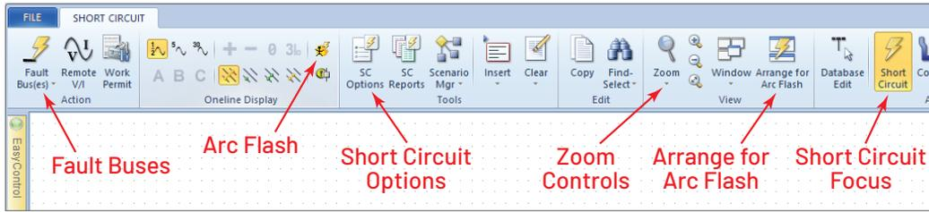
Figure 8.52: Short Circuit Tab Options
