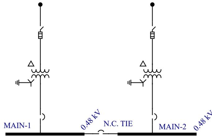
Figure 5.2: Double-End Load Center Configuration
