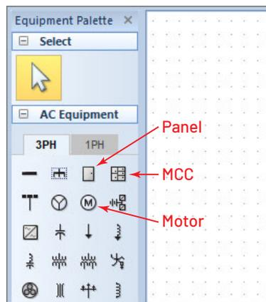
Figure 8.13: Panel, MCC, and Motor Icons on the Equipment Palette
