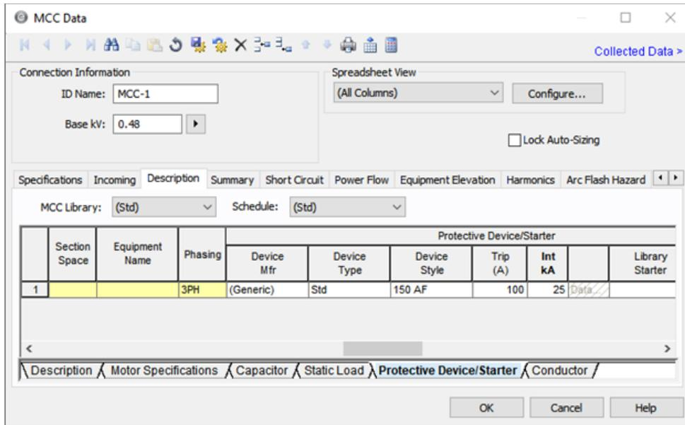
Figure 8.34: MCC Description Tab, Breaker Specification
