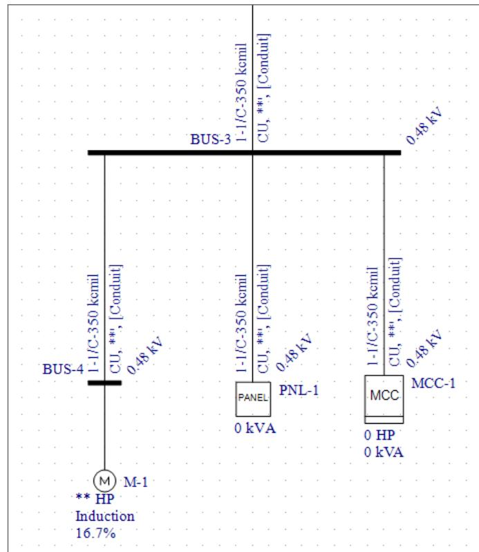
Figure 8.14: Motor, Panel, and MCC are Connected
