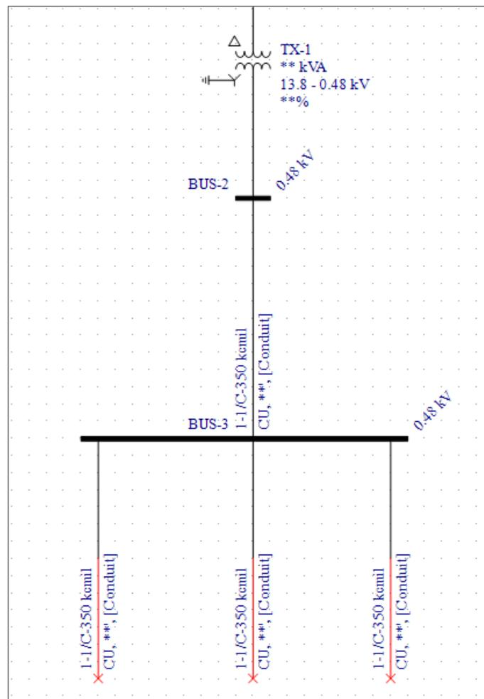
Figure 8.11: Three Cables Connected
