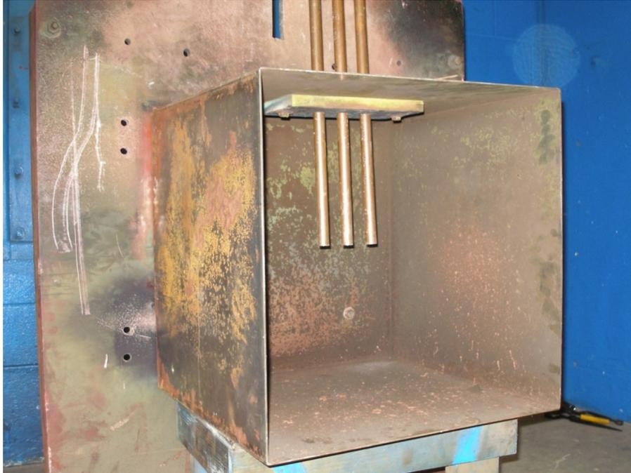
*Figure 3.5 – IEEE 1584-2002 Test Setup*
