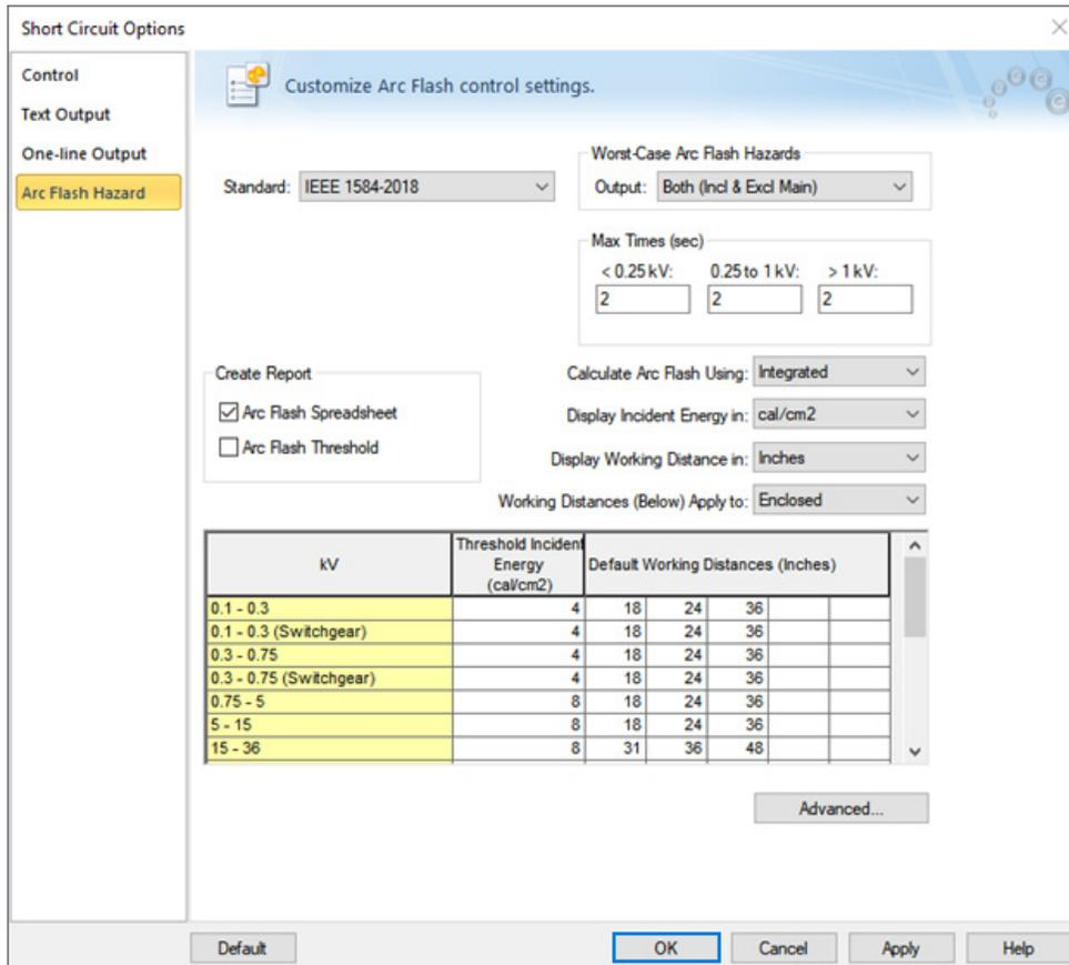
Figure 8.54: Short Circuit Options – Arc Flash Hazard Tab
