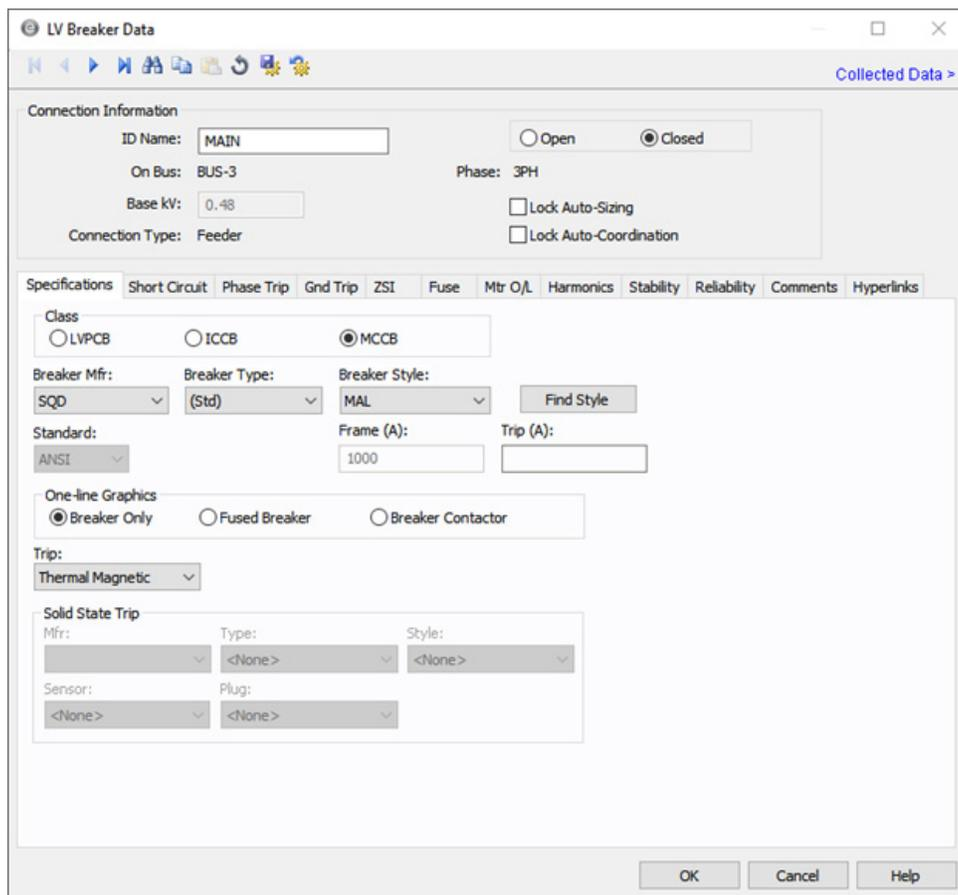
Figure 8.37: Main Breaker, Specifications Tab
