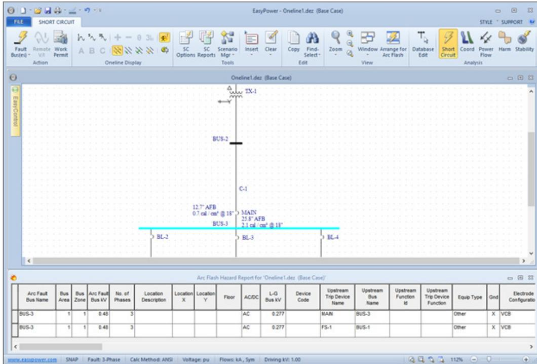
Figure 8.55: Arc Flash Results with the Arc Flash Hazard Report Displayed
