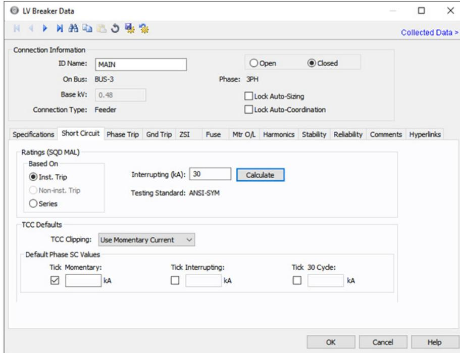
Figure 8.38: Main Breaker, Short Circuit Tab
