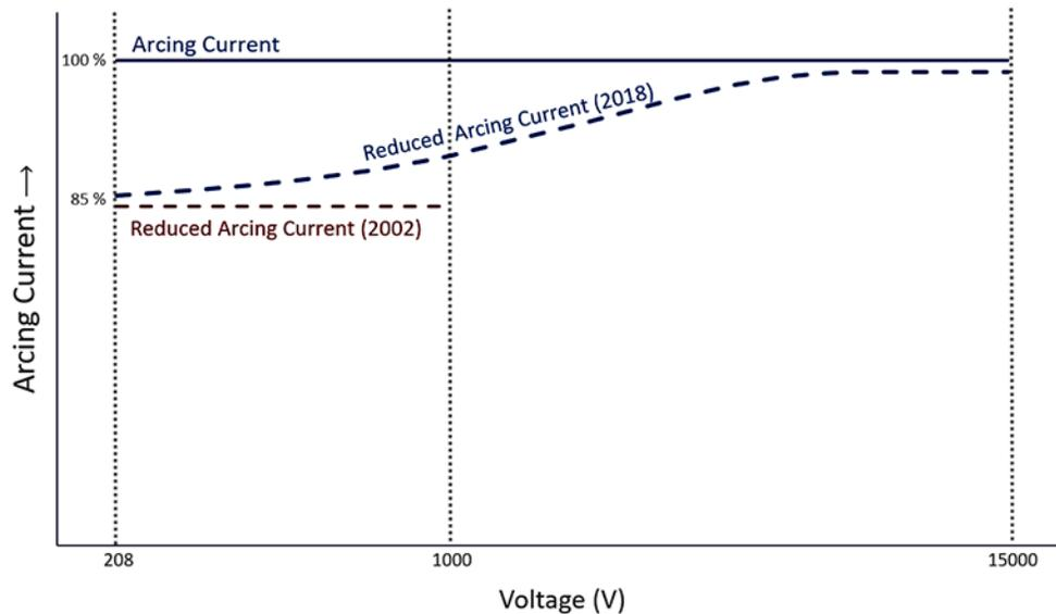
*Figure 3.2: Reduced Arcing Current*
