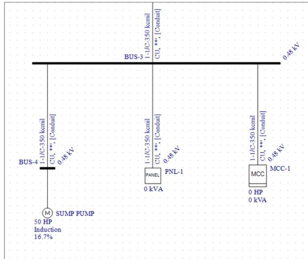
Figure 8.18: Data Displayed on Motor
