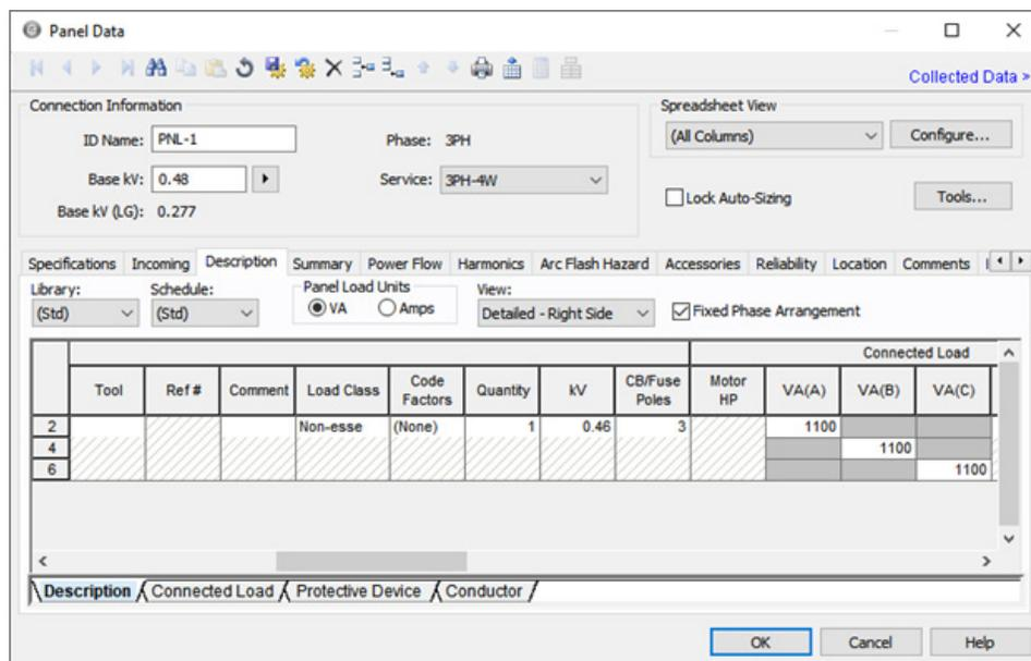
Figure 8.27: Connected Load on the Description Tab
