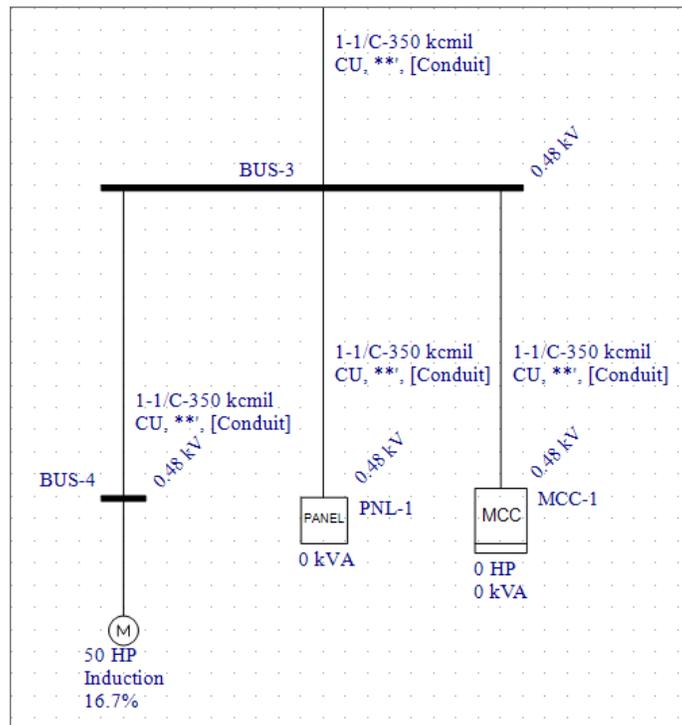
Figure 8.19: One-line that Reflects Text Visibility Settings
