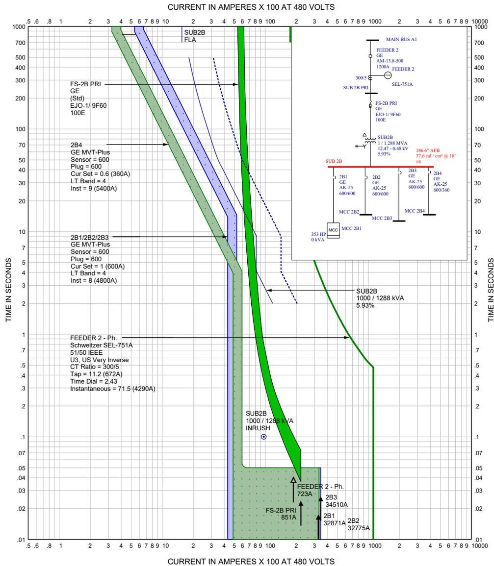
Figure 5.4: Feeder 2 Relay Normal Settings – Arc-Flash at Sub 2B Bus – 37.4 cal/cm<sup>2</sup>
