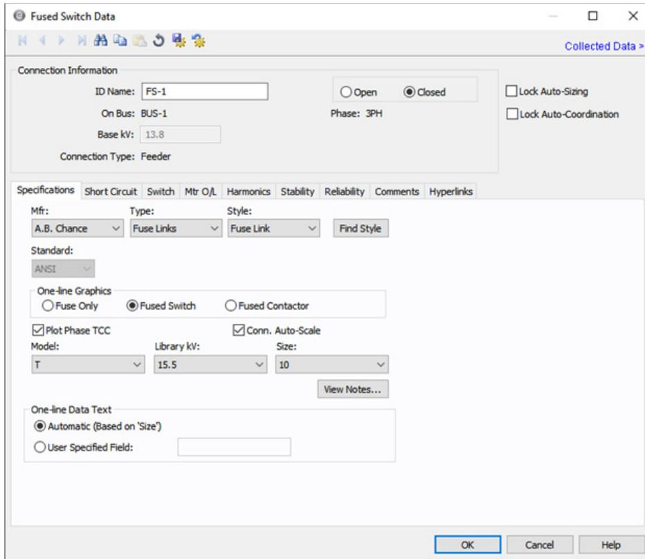
Figure 8.47: Fused Switch Data – Specifications Tab
