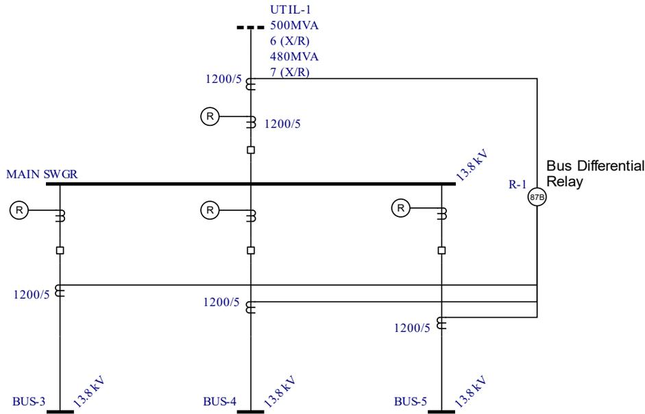
Figure 5.8: Typical Bus Differential Relaying System
