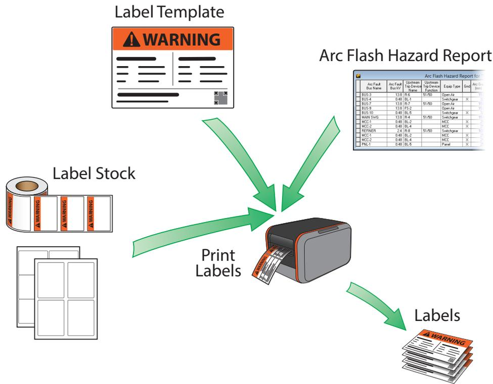
Figure 9.5: Arc-Flash Label Printing Workflow
