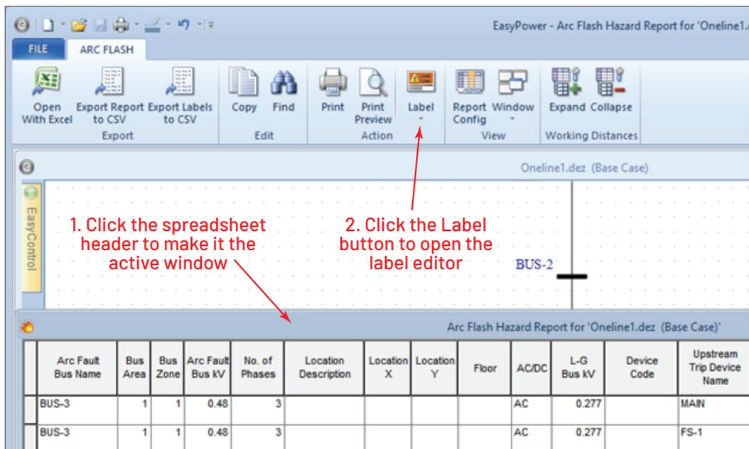
Figure 8.56: Printing Arc Flash Hazard Labels
