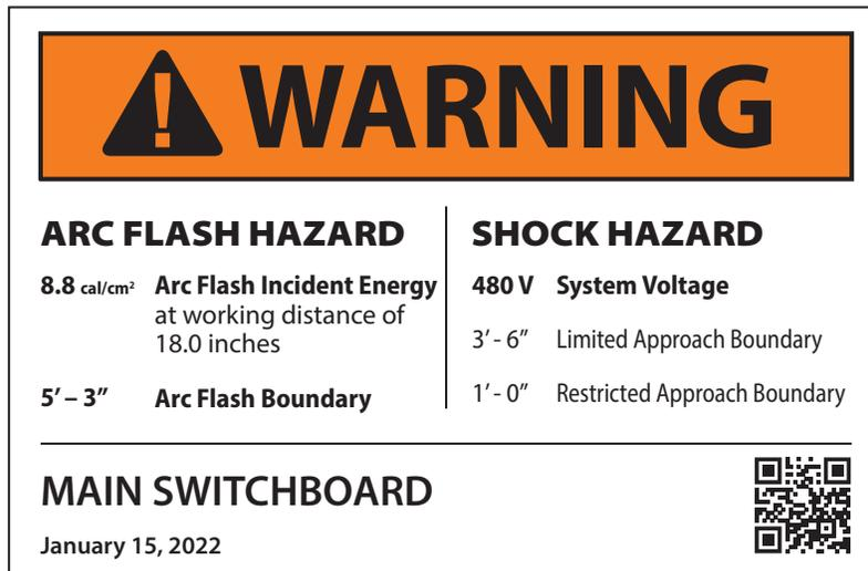
*Figure 9.3: ANSI Z535 Arc-Flash Label Example*
