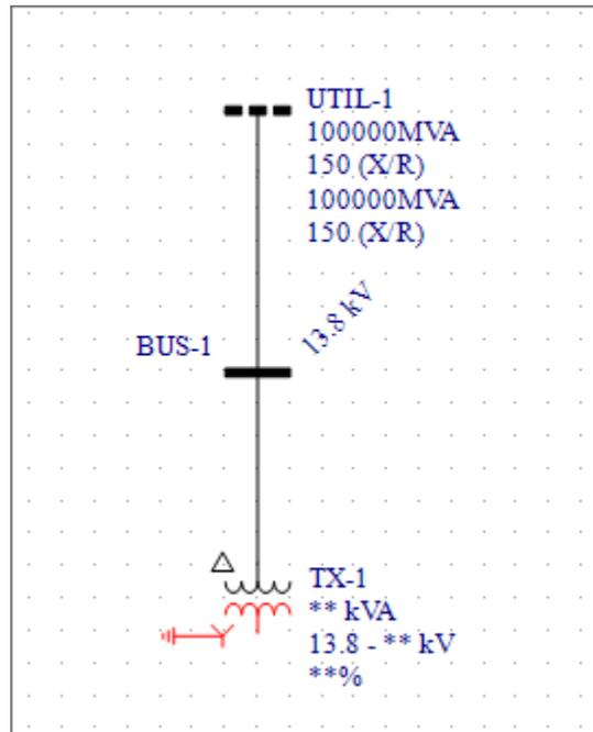
Figure 8.6: Two-Winding Transformer is Connected to the Utility
