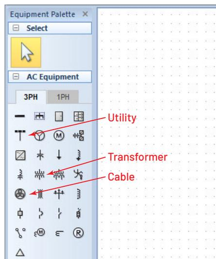
*Figure 8.3: Icons for a Utility, Transformer, and Cable on the Equipment Palette*
