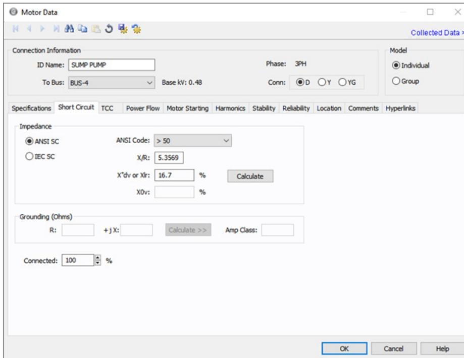
Figure 8.17: X/R Calculated in the Motor Short Circuit Tab
