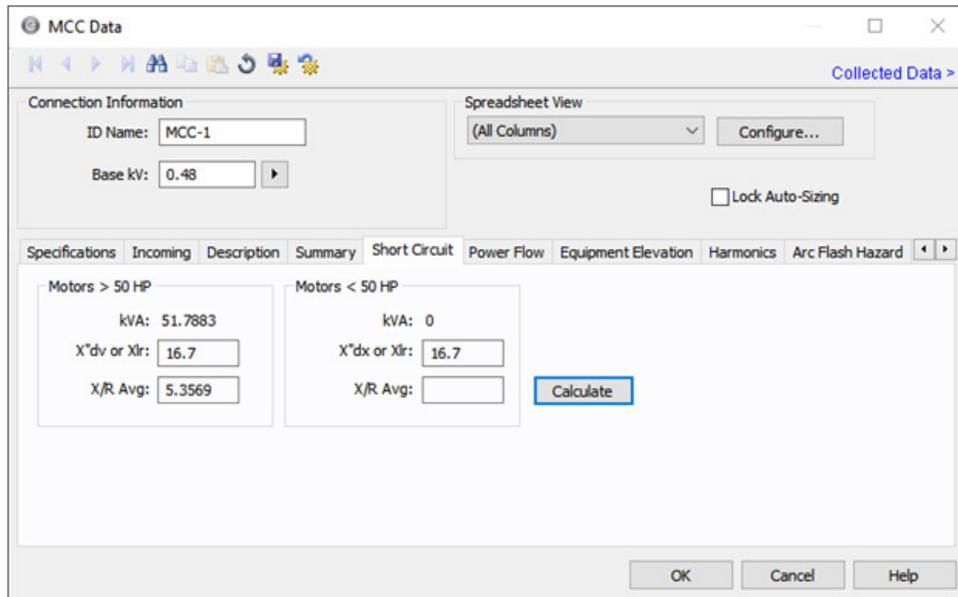
Figure 8.36: MCC Short Circuit Tab, Calculate X/R Average
