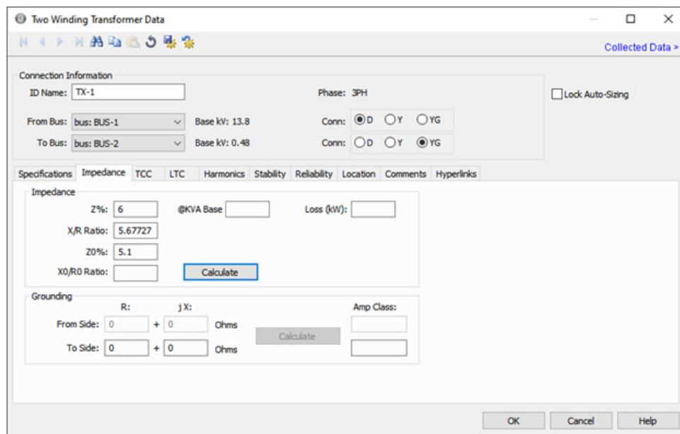
Figure 8.45: Transformer Data – Impedance Tab
