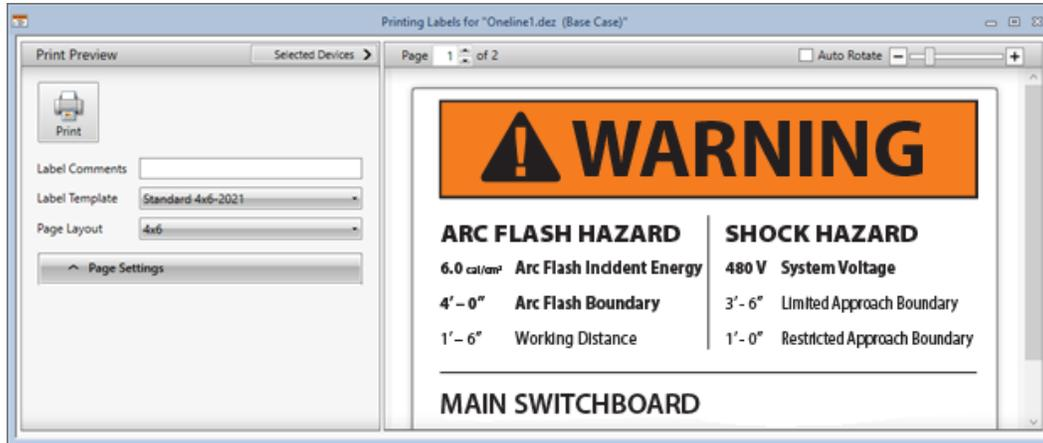
Figure 8.57: Printing an Arc Flash Hazard Label
