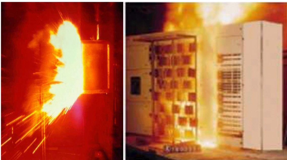
*Figure 2.1: (a) Arc Blast in Box; (b) Arcing Fault in an Electrical Panelboard*
