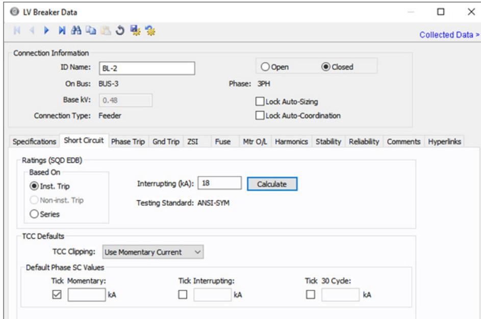
Figure 8.41: Feeder Breaker – Short Circuit Tab
