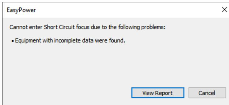
Figure 8.50: Dialog Box Indicating Errors Due to Missing Data
