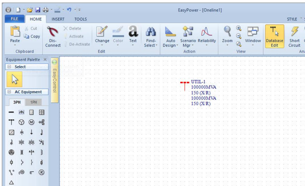
Figure 8.4: Utility Placed on the One-line Drawing
