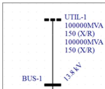
Figure 8.48: Utility Data, Infinite Source
