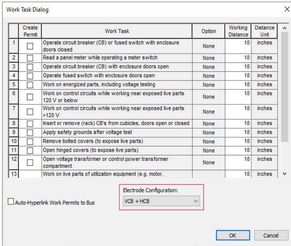
Figure 3.11 – Selection of Electrode Orientation, Within the Energized Work Permit Dialogue Box
