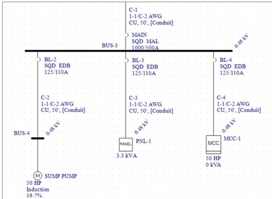
Figure 8.43: Data Entered for Loads, Cables and Breakers
