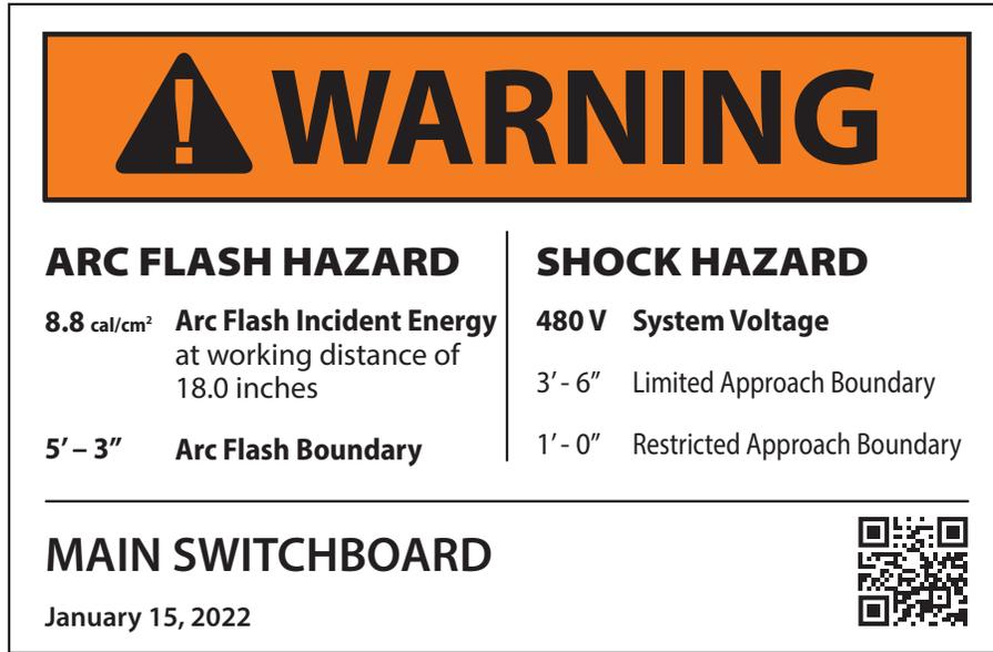
Figure 4.5: Example of an Arc -Flash Warning Label Created by EasyPower
