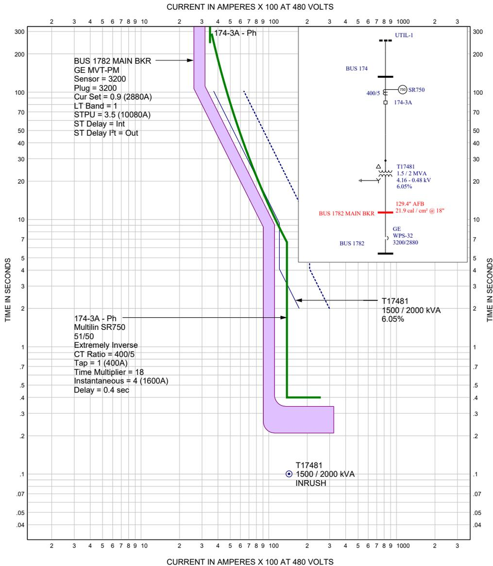
Figure 5.10: Typical Time Overcurrent Curve for a Transformer Primary Relay (Revised)
