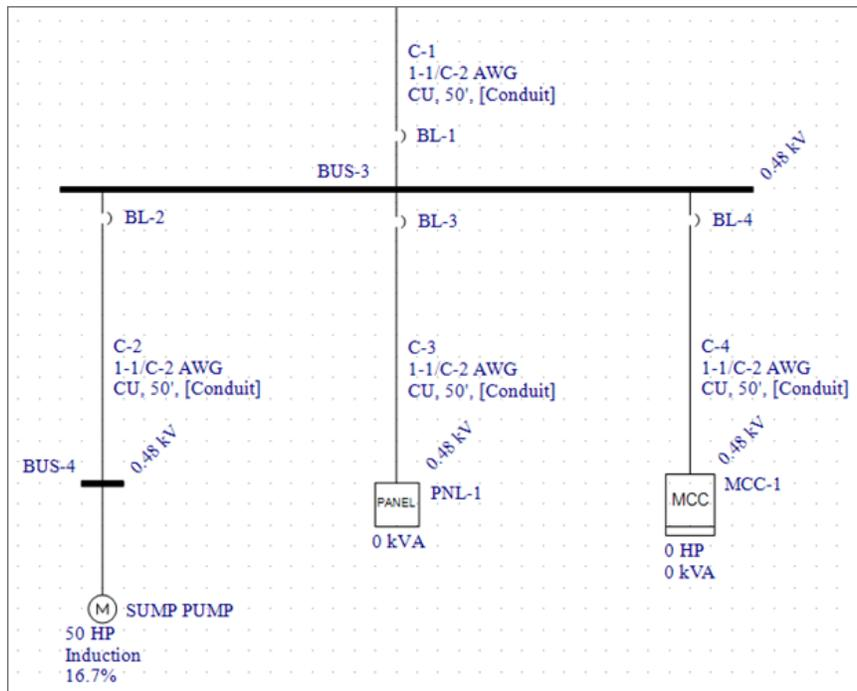
Figure 8.23: One-line Display After Copying and Pasting the Cable Information
