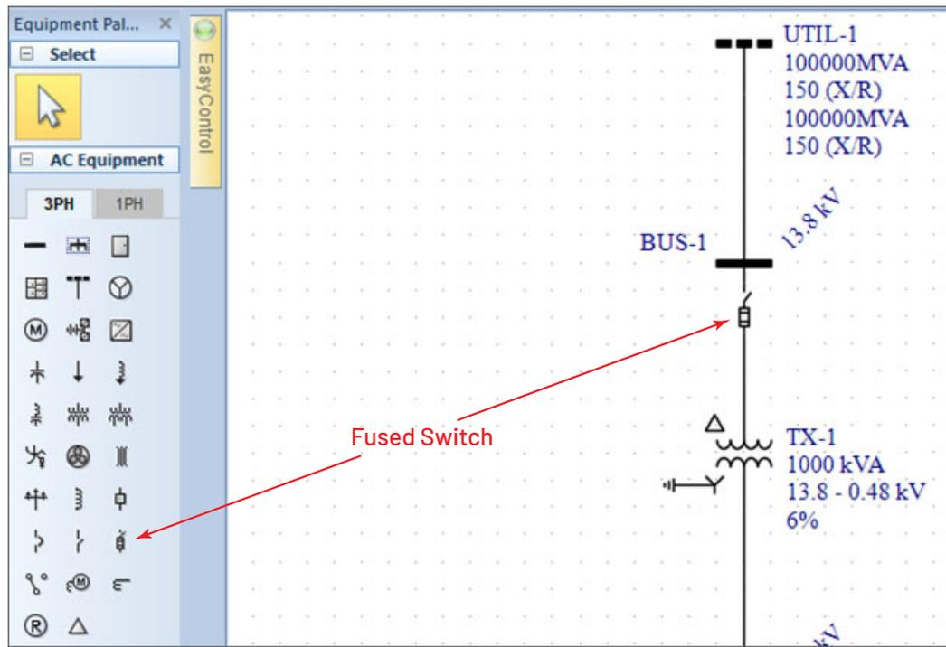
Figure 8.46: Correctly Place Fused Switch (FS-1)
