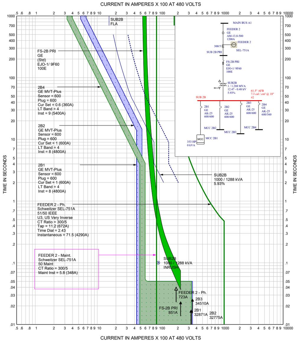
Figure 5.5: Feeder 2 Relay in Maintenance Mode – Arc-Flash at Sub 2B – 7.3 cal/cm<sup>2</sup>
