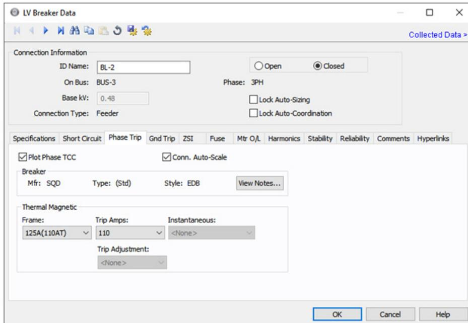
Figure 8.42: Feeder Breaker – Phase Trip Tab
