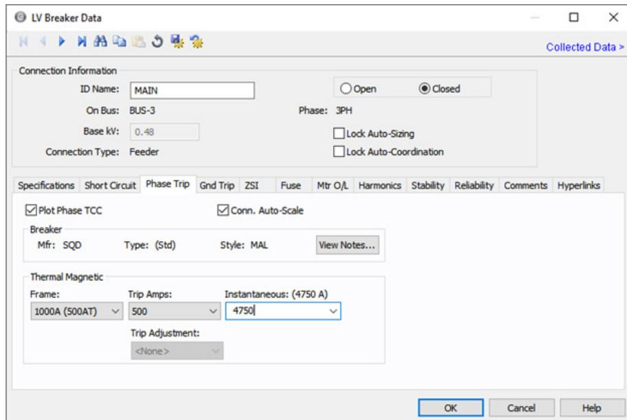
Figure 8.39: Main Breaker - Phase Trip Tab
