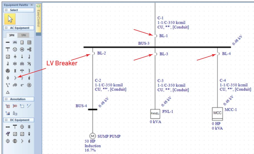
Figure 8.21: Adding Breakers
