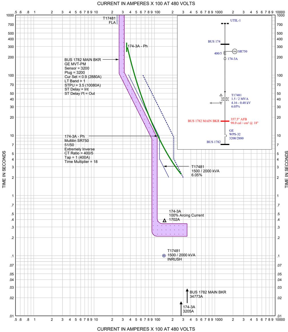
Figure 5.9: Typical Time Overcurrent Curve for a Transformer Primary Relay
