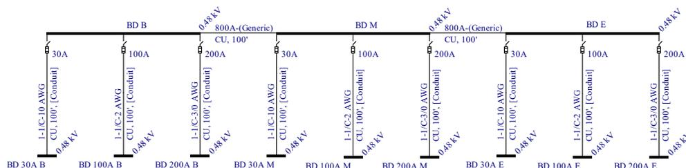
Figure 7.1: Generic Bus Duct Example
