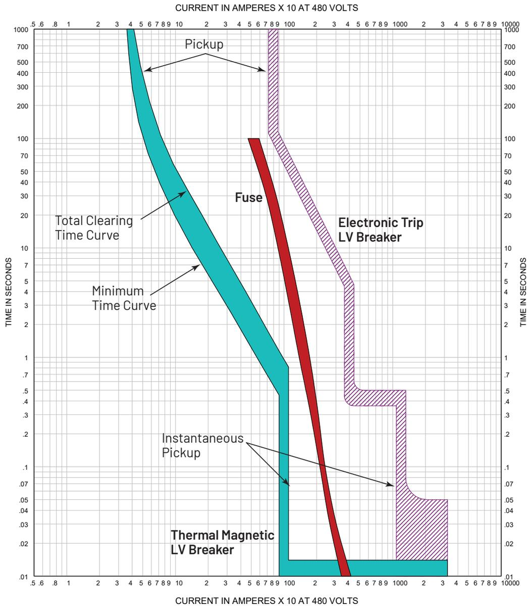
Figure 4.2: Example of TCC Plot with Tolerance Band
