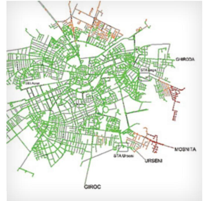
Aquatim SA was tasked with stepping up its hydraulic modeling for the water distribution network in Timișoara, located in western Romania. The USD 200,000 project involved modernizing its digital infrastructure by importing data into a model for easier visibility. The team used OpenFlows to connect the main distribution network to the GIS system and extended the model. The application helped Aquatim
